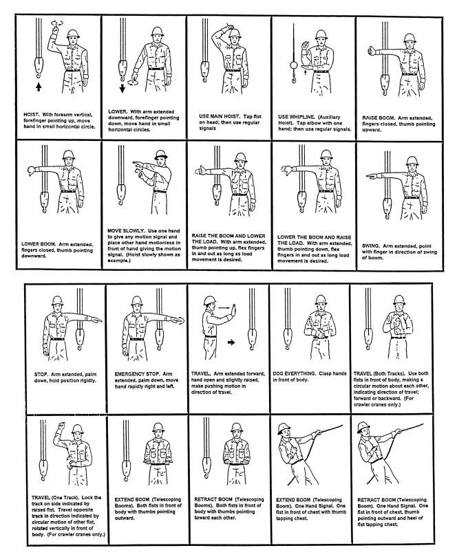
STANDARD HAND SIGNALS FOR CONTROLLING OVER-HEAD AND GANTRY CRANES
